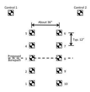
Figure 1. Typical Arrangement of Targets on Each Site
